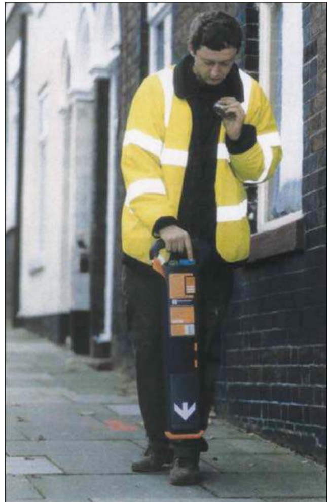
Figure 5 Using a cable locator
