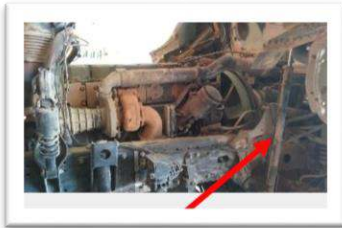
Hydraulic cylinder in situ
