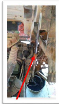
Hydraulic cylinder broke at this point
