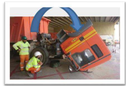
Cab fell forward onto ground
