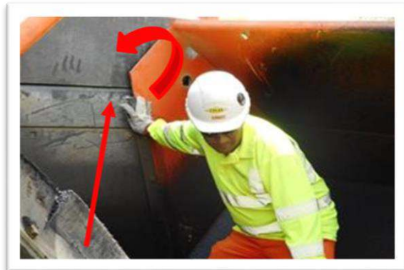
2. Finger crushed by hopper wing
