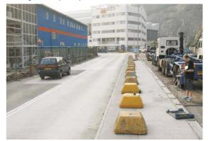
The tests were carried out on a low speed, smooth, worn concrete road with a speed limit of 60 km/hour, conditions which would in theory give a relatively low expected noise reduction. A vehicle was driven over both treated and untreated areas of the road during periods of low ambient noise with the noise levels being measured and recorded in decibels.
